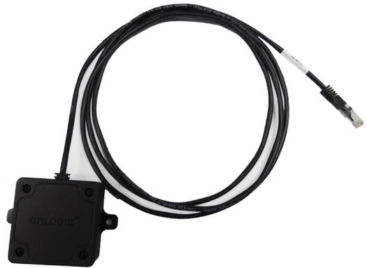
Enlogic's Spot Fluid Leak Sensor is designed to reliably monitor a remote location for the presence of water or any other conductive liquid (with resistivity of less than 2M ohms per cm). The sensor can be extended (up to 30.5 m) using a standard RJ-45 coupling.
