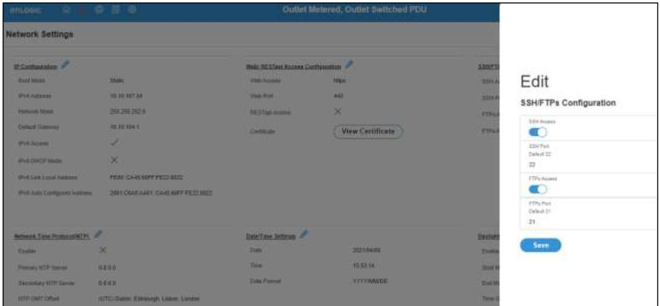
Figure 15: SSH/FTP Configuration
