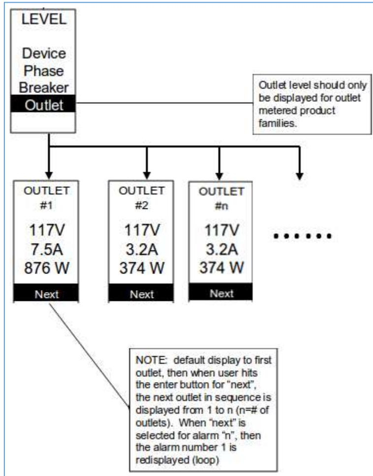
**Note:** Custom outlet names noted in the WebGUI do not make changes to the local display. This is done to make it easier to map to outlet numbers which can locally be seen on the outlets themselves.
