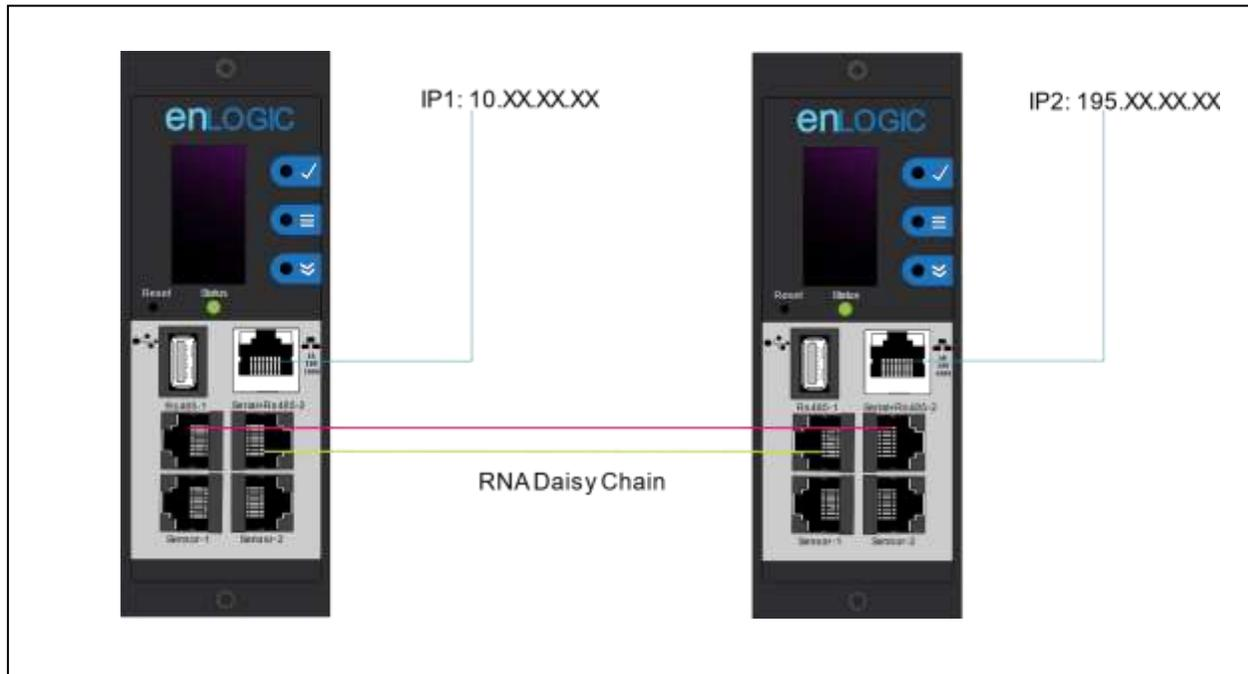
Figure 51: Connection Diagram RNA Daisy Chain
