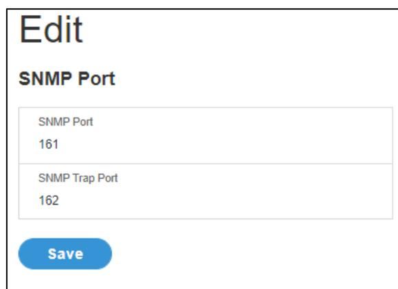
The image shows a web interface window titled "Edit SNMP Port". It contains two input fields: "SNMP Port" with the value "161" and "SNMP Trap Port" with the value "162". A blue "Save" button is located at the bottom of the form.
