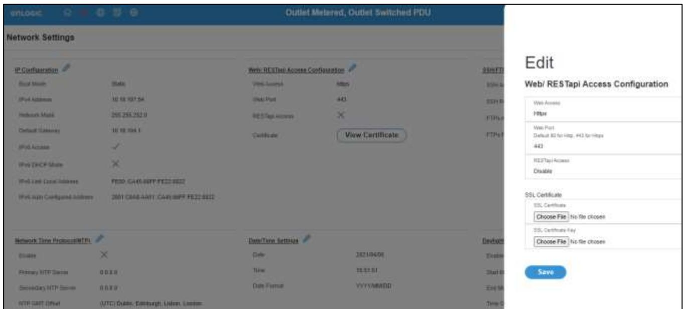
Figure 14: Web RESTapi Access Configuration can be used to set HTTP, HTTPS or Disable the onboard Web GUI.
