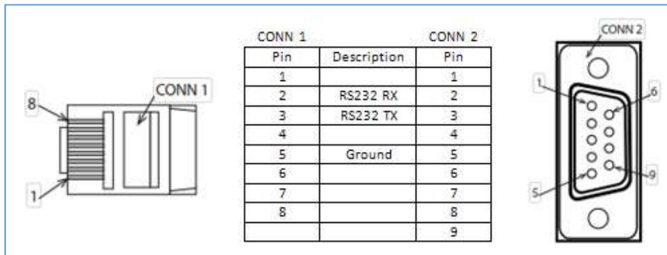
Figure 58: Serial Cable Pinout
