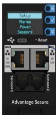
Reset Key Button : Use this recessed Pin hole for the Reset functionality.
