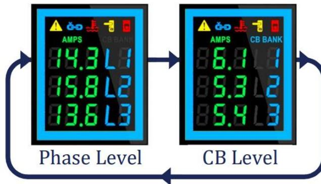
The Seven Segment LED display shows data in high visibility at Phase Level and CB Level.
